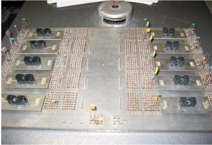
Burn-in Board used for Dynamic Life Test
