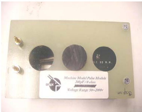
Back view of the ESD tester with Machine model/Pulse model being used
