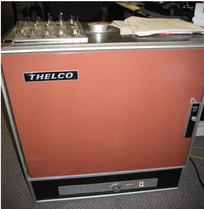
Burn-in oven used for Dynamic Life and Humidity Test
