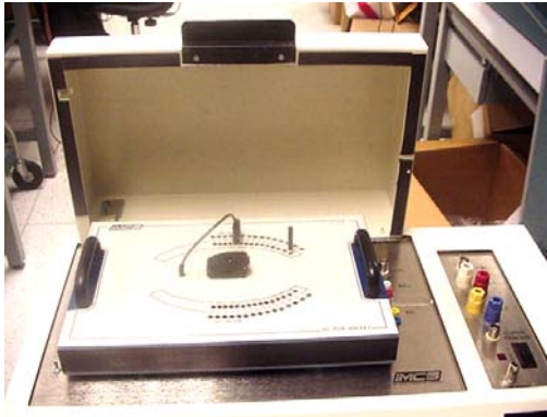
Front view of the iMCS model#700 ESD tester with lid open
