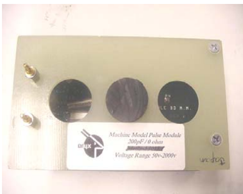
Back view of the ESD tester with Machine model/Pulse model being used
