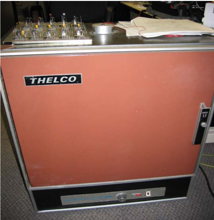
Burn-in oven used for Dynamic Life and Humidity Test
