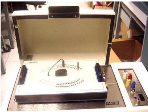
Front view of the iMCS model # 700 ESD tester with lid open
