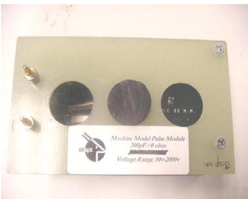
Back view of the ESD tester with Machine model/Pulse being used.
