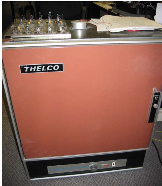
Burn-in oven used for testing
