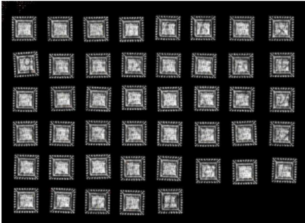
Package Type: QFN 32L (5*5) After Pre-con LEVEL 3 Photo no : Fig 2 Die Surface SAT Result : 0/45ea dalam =>PASS.
