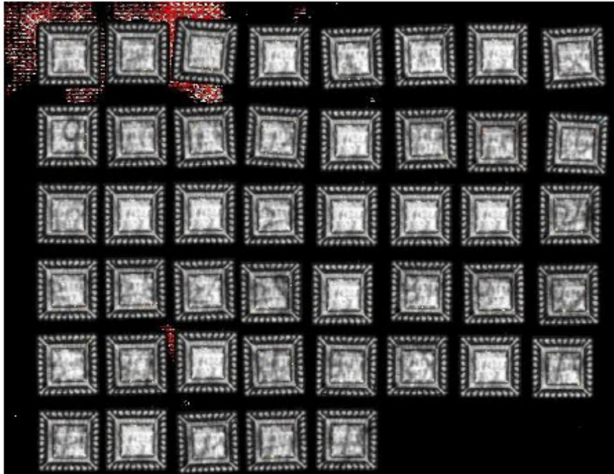
Package Type: QFN 32L (5*5) Before Pre-con LEVEL 3 Photo no : Fig 1 Die Surface SAT Result : 0/45ea delam =>PASS.
