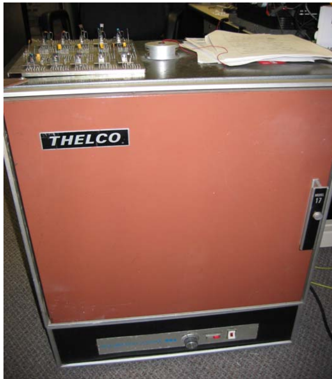
Burn-in oven used for testing
