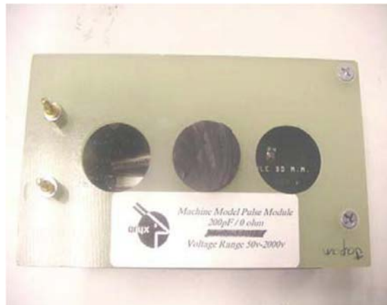
Back view of the ESD Tester with the Machine Model/Pulse Model being used
