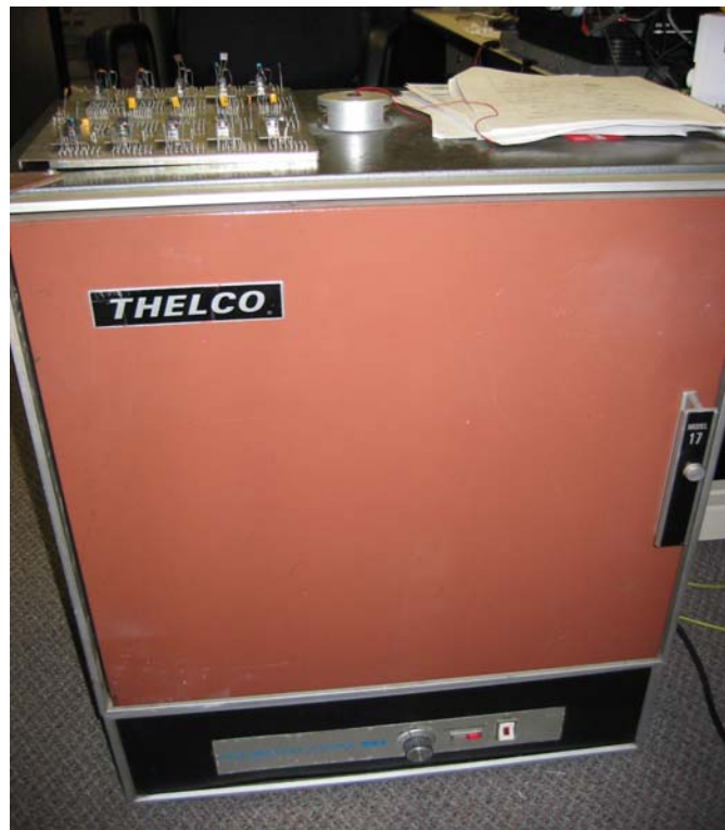
Burn-in oven used for testing
