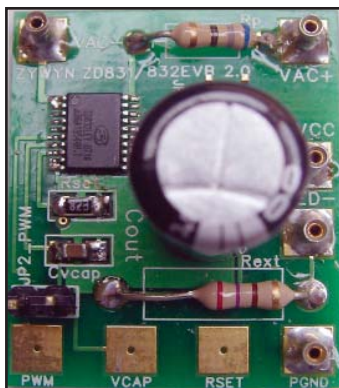
Figure 8. ZD832EVB evaluation board configured for 240V_{AC} operation.
